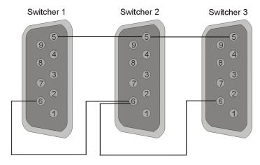
More specifically, the output of one switcher is connected to INPUT 6 of the next switcher. Once loop control is enabled these switchers will automatically switch video signals to the output of the second switcher through INPUT 6. Keep in mind that you are always going to have one less input than the total number of inputs available on all switchers. The figure above is for an 11-in 1-out switcher.
